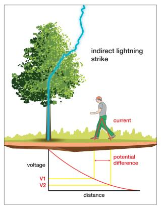
If lightning strikes nearby, the voltage dissipates with increasing distance from the point of the strike.
